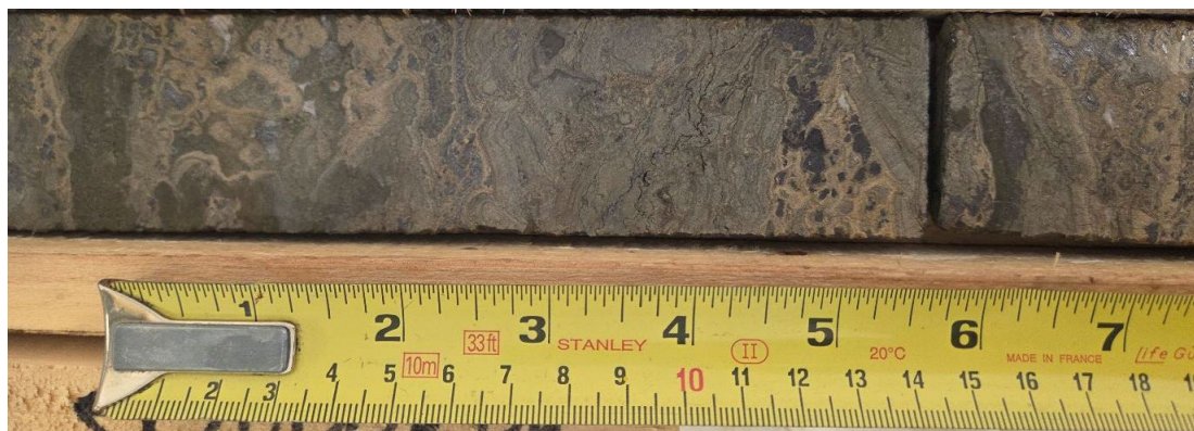
Photo of part of sulphide intercept in 3312-104 showing banded sphalerite. Part of an assay interval of 1.90m grading 32.08% Zn, 11.84% Pb, 105g/t Ag.
